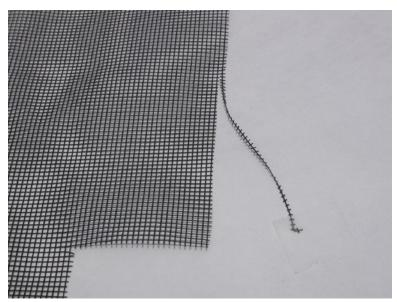
Figure 4. Nylon mesh and one strand partially cut.
