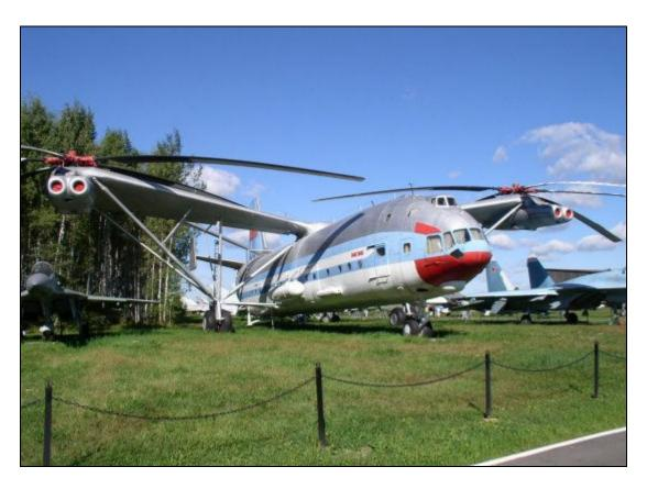
This helicopter is the largest helicopter ever built. It is the Soviet Mil V-12. It was developed in the 1960s. The distance from the edge of one of rotor disk to the other was 220 feet, which is wider than a Boeing 747. Two V-12 prototypes were built, but the design was too big and difficult to maneuver to be practical.
